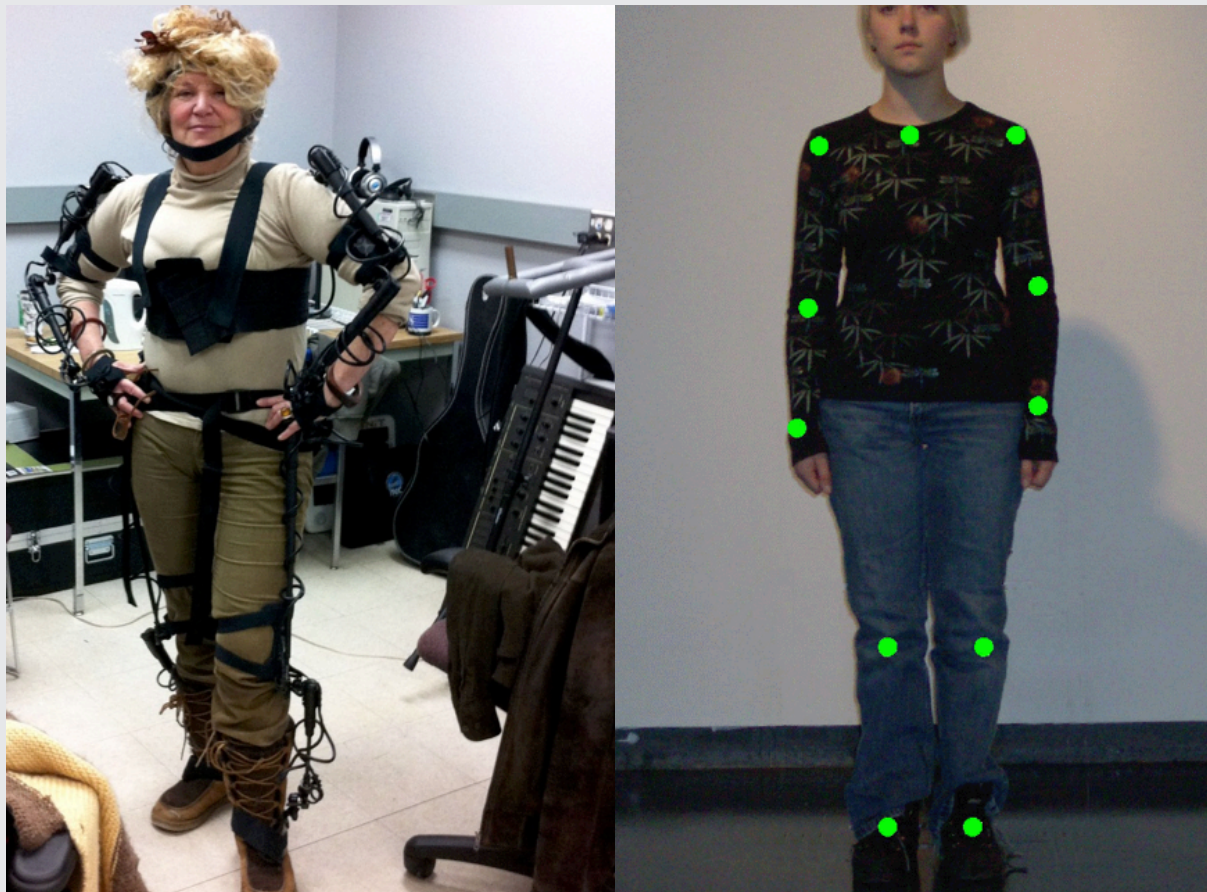
Figure 10-6: (Left) Gypsy 6 motion capture suit uses mechanical and inertial devices to capture joint positions and send them by wireless link to a computer. (Right) Optical motion capture systems instrument the actor with small targets, often balls of a known colour
