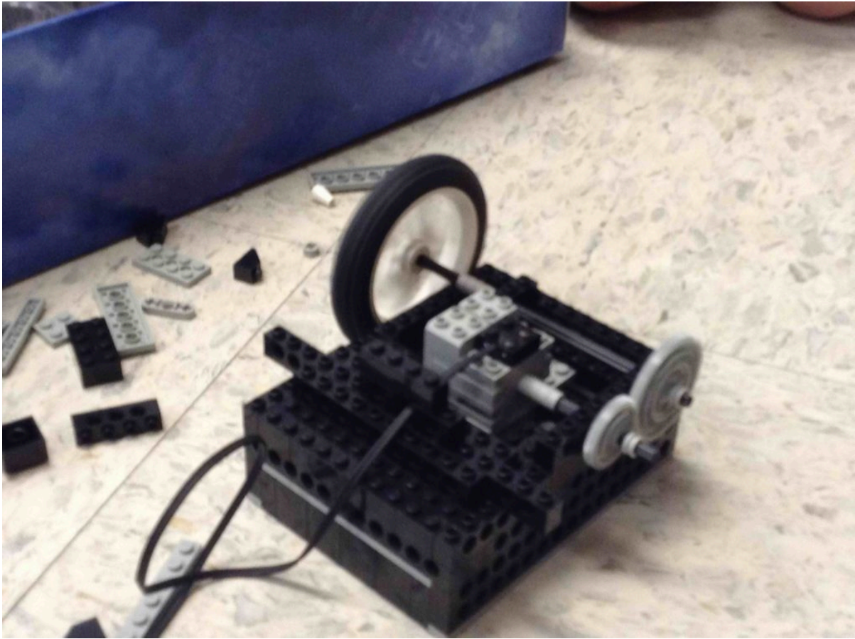
Figure 6. A simple gear train to achieve maximum speed.
