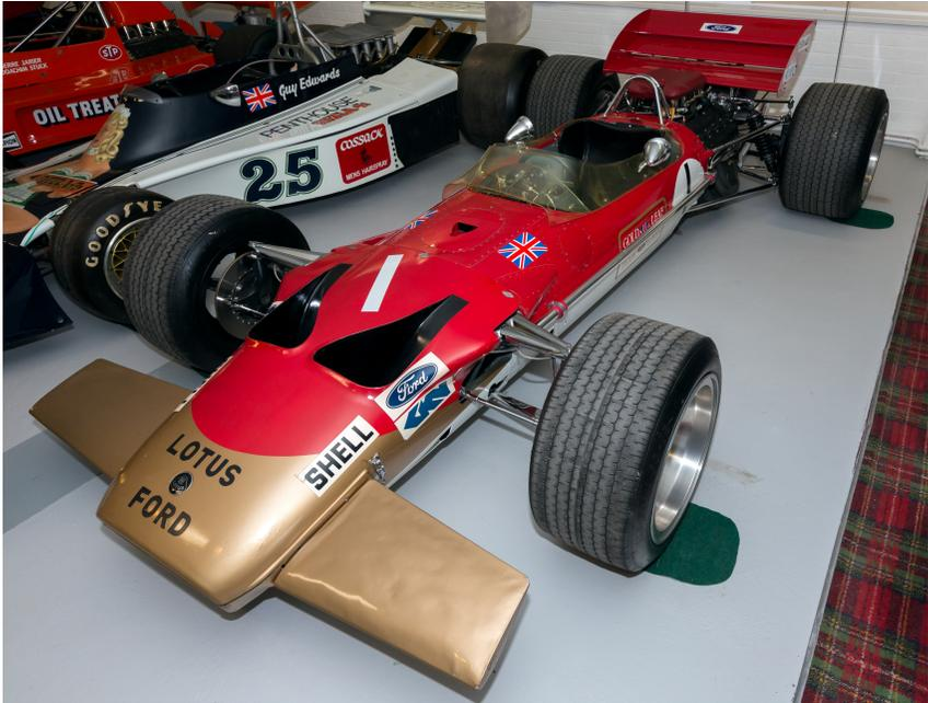
Figure 1. The Louts 49B features front and rear wings. (Credit: Morio)
