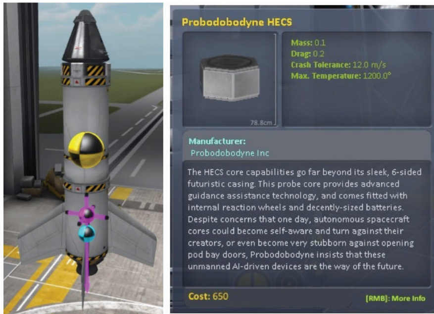
Figure 4: A visualization of the center of mass, thrust and lift on a rocket (left) and detailed information about the properties which combine to create those (right).
